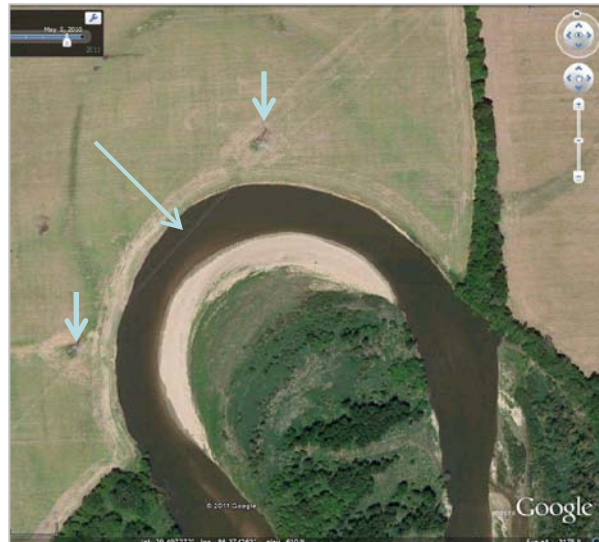
Figure 4. Same White River location near Centerton, IN (2010). The lines now run over the active channel and the utility poles are at risk from future erosion.
